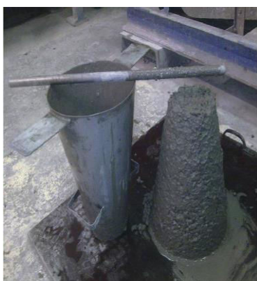
Fig 7: slump cone test apparatus
